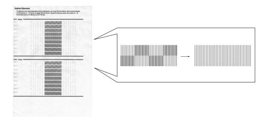
**3** Select the best aligned print sample (1 to 9) for 360 and 720 dpi by using the Up/Down scroll control.
